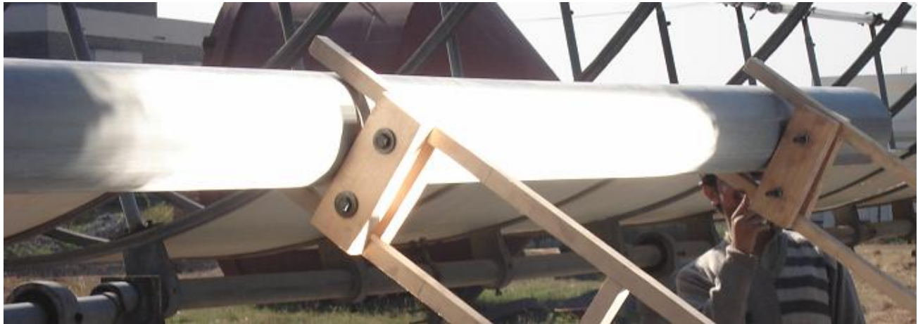
Figure: The Accuracy of the Focal point of SPC-24 being evaluated. The Temperature at the focus was around 365 degree Celsius.
